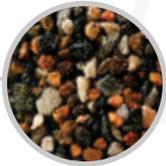
Fine cast of sand applied to assist with slip resistance
